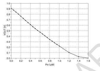
Output Voltage (OUT) vs. Input Power, Fin= 61.5 GHz
